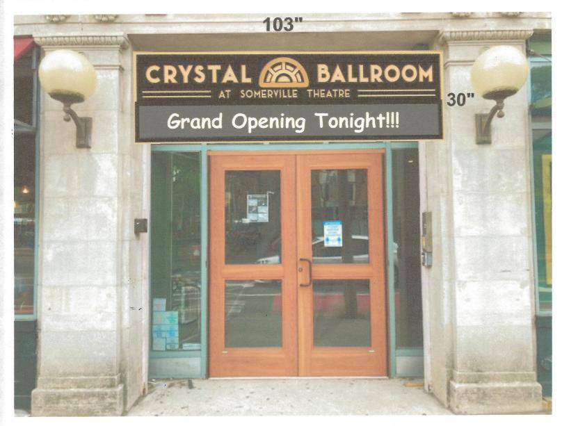
Propose to install one (1) new single faced illuminated sign/digital reader board for recessed area above doors. Overall size is 30" x 103" x 12" in depth, with "Crystal Ballroom" illuminated with exposed white LED lamps and accent lines and AT SOMERVILLE THEATRE having push thru halo lighting. Reader Board is 12" high with possible changing message and graphics for Theatre and Community messages.
